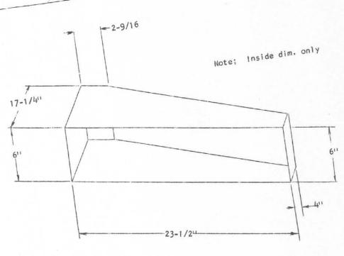
Detail For Placement of Mounting Holes in Bottom Board
